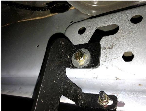
**Step 11.** After final adjustment, tighten all three brackets at the main tube.
