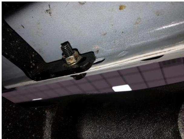
**Step 9:** Begin tightening the lower attachment points starting with the rear bracket working your way up to the front bracket. ( **20ft/lbs** )
