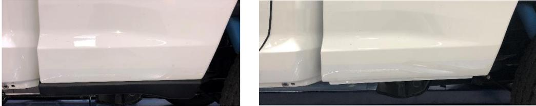
**Step 7:** Carefully place step into position and start the upper 3/8"X1" hex bolt and 3/8" flat washer in the center bracket and hand tighten to hold in place. Next, install the remainder 3/8"x1" hex bolts and 3/8" washer in the front and rear brackets and leave loose for now.
