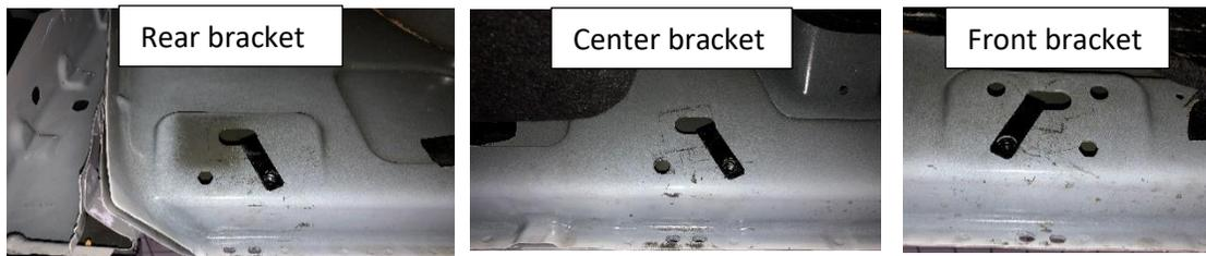
U-clip positioning. **NOTE: Clip orientation will be the same for passenger side.**
